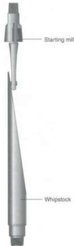
Figure 5 - Starting mill pinned to the whipstock
