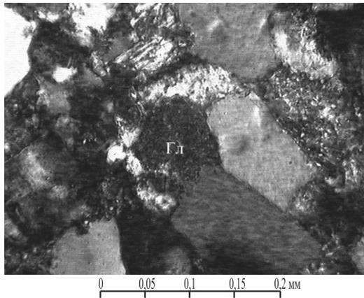
**Fig. 8.** Glauconite (Gl). Contact cementation of fragments. The microsection, 2 nic., depth 3074,1 m
