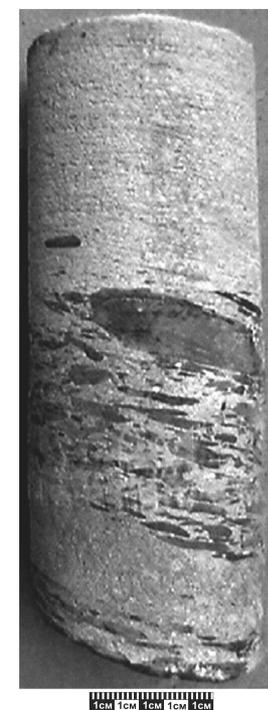
**Fig. 3.** Shift deformation of laminae in clay-siltstone interstratification. The core, depth 3066 m
