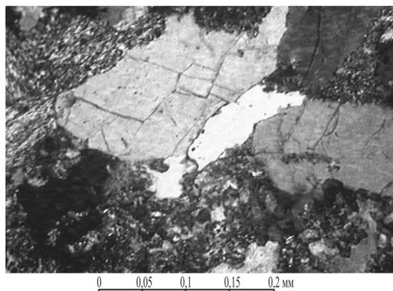
**Fig. 6.** Grains of fissured quartz. The microsection, 2 nic., depth 3131,3 m
