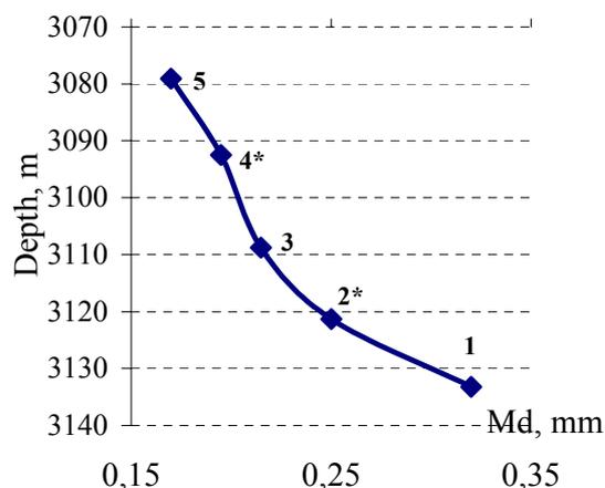
**Fig. 4.** Change of grain's median diameter (in microsections) according to cyclitis  $J_{15}$  cut
