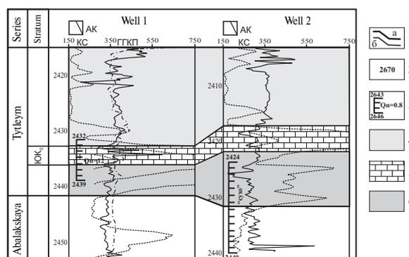
Fig. 1. Lithologo-geophysical cuts of the Tutleym series: 1) series borders (a), layers (b); 2) cable depth, m; 3) an interval of approbation and test results in the punched stem:  $Q_n$  – oil debit,  $m^3/day$ ; deposits: 4) clay-siliceous bituminous, 5) carbonate, 6) kaolinite-clay
