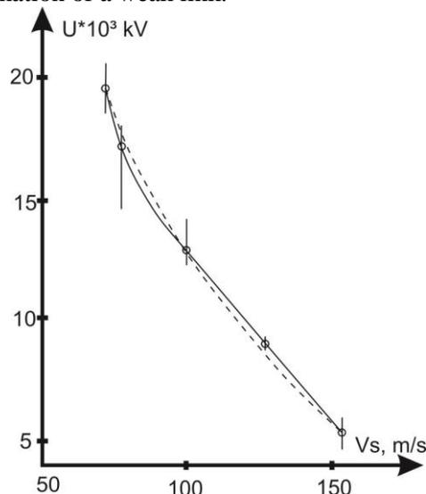
**Figure 4.** Dependence of breakdown voltage gap on the transformer oil flow rate.
