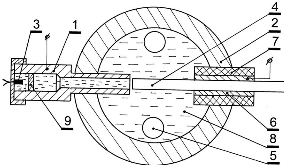
**Figure 3.** Contact system of the high-voltage explosive switch model, where 1 is explosion chamber; 2 is arc-extinguishing chamber; 3 is explosive charge; 4 is movable rod; 5 is pocket air; 6 is guide, 7 is insulator; 8 is transformer oil; 9 is piston.
