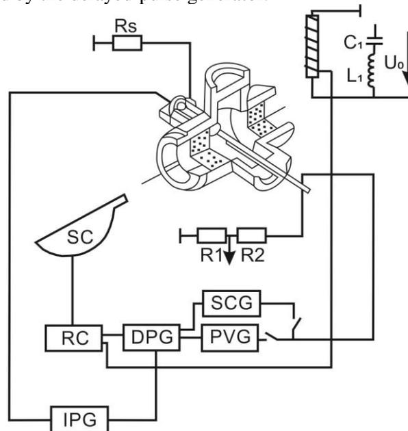
**Figure 2.** Flow chart of the installation, where SCG is surge-current generator; PVG is pulsed-voltage generator; IPG is initiating pulses generator; DPG is delayed-pulse generator; SC is streak camera;  $R_1$ ,  $R_2$  are a voltage divider;  $R_s$  is shunt;  $C_2$ ,  $L_2$  are backlight supply; RC is remote control.
