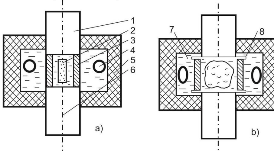
**Figure 1.** Explosive switch in its initial condition.
