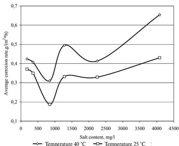
**Fig. 2.** Dependence of corrosion rate of carbon steel (St. 3) in circulating water of modeling WRC on salt content of makeup water
