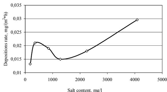
**Fig. 3.** Dependence of depositions rate in circulating water of modeling WRC on salt content of makeup water
