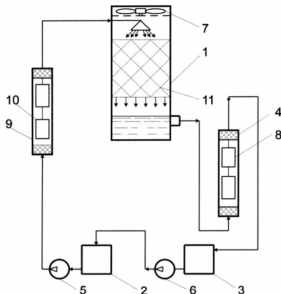
**Fig. 1.** The diagram of the laboratory setup, modeling the system of the reverse water supply: 1) the tower-cooler; 2) the capacity with a heater (thermostat); 3) the capacity of chilled water; 4, 9) the glass tube for check samples set up; 5, 6) the pump; 7) the fan; 8, 10) the check samples for research the rate of corrosion, depositions of salts and fouling; 11) the head of Rashing ring
