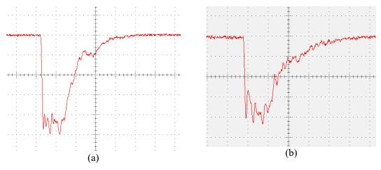
Figure 6. Oscillograms of output pulses at different switching conditions, (a) in argon; (b) in argon with 5-7% insulating gas.
