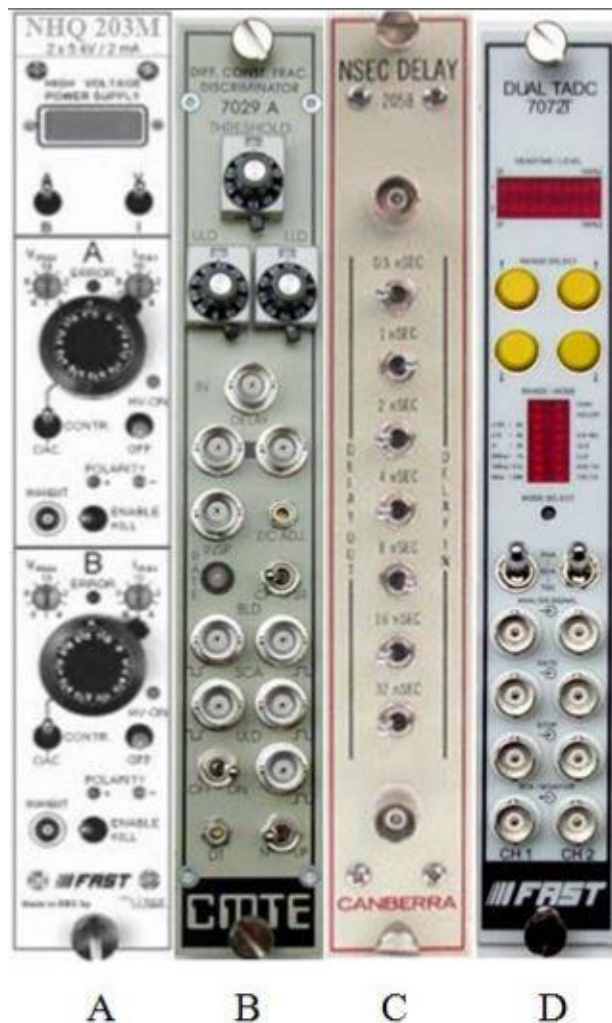
Figure 8 – A – high voltage power source B – a differential discriminator, C – block nanosecond of delay, D – time-to-digital converter.
