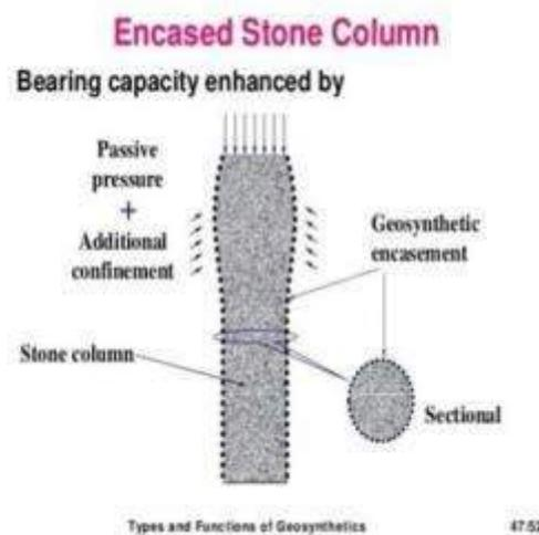
Figure 8. Encased Stone Column
