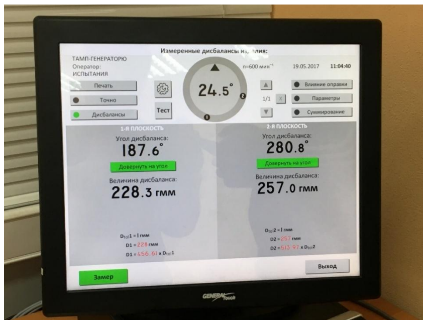
Pic.28 Initial imbalance A and B
