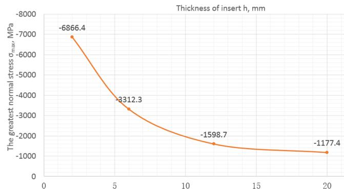
Fig. 9. Influence of the cutting insert thickness on the maximum value of the principle normal stress in the cutting wedge
