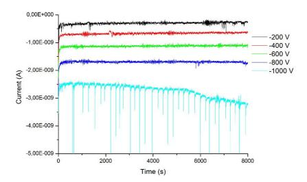
Fig. 2. The measurements of the produced current when the detectors are irradiated by  $\beta$ -particles of Sr with a negative voltage applying.
