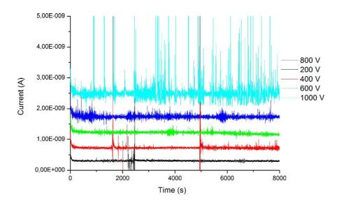
Fig. 1. The measurements of the produced current when the detectors are irradiated by  $\beta$ -particles of Sr with a positive voltage applying.
