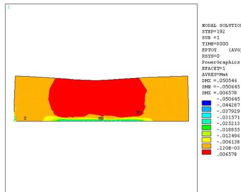
Fig.3. The residual strains  $\epsilon_y$
