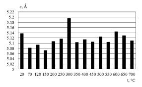
Fig. 2. The dependence of the parameter c of zirconium alloy Zr-2.5Nb from temperature.
