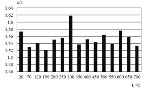
Fig. 3. The ratio *c/a* of zirconium alloy Zr-2.5Nb.
