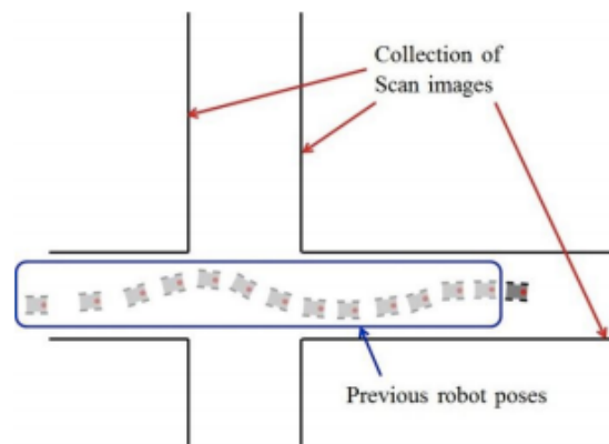
Figure 4. Scan-based map is a collection of raw scan images and corresponding robot poses
