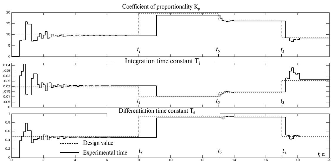
Fig. 5. Diagrams of determination of PID-regulator parameters (where  $t_1$ ,  $t_2$ ,  $t_3$  are the moments of CO nonstationarity occurrence)
