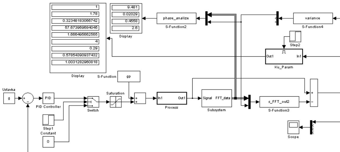
Fig. 3. The model of the adaptive system with frequency division of control and self-adjustment channel in Simulink (Matlab) medium
