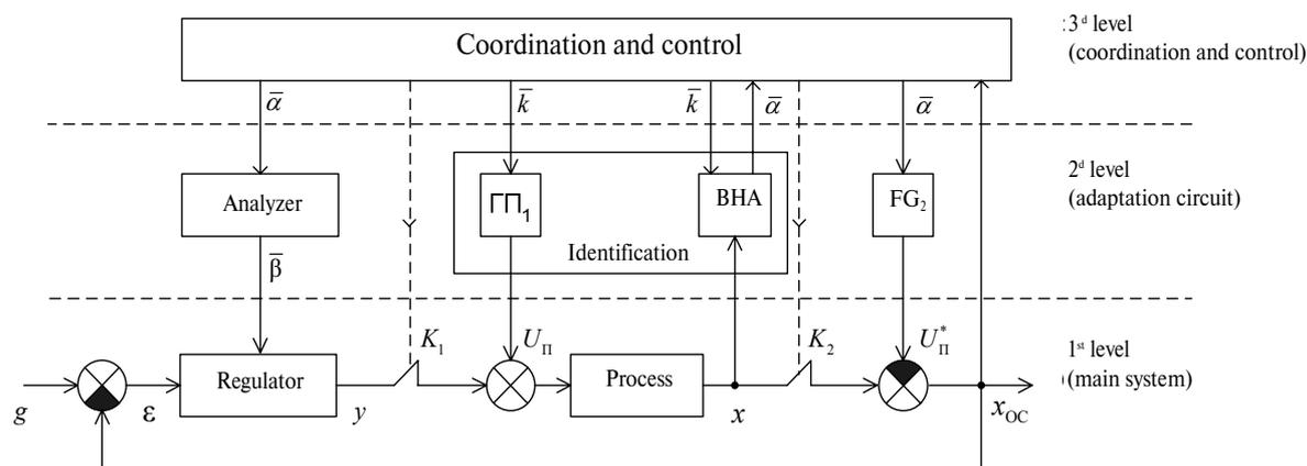
Fig. 1. Block diagram of adaptive system
