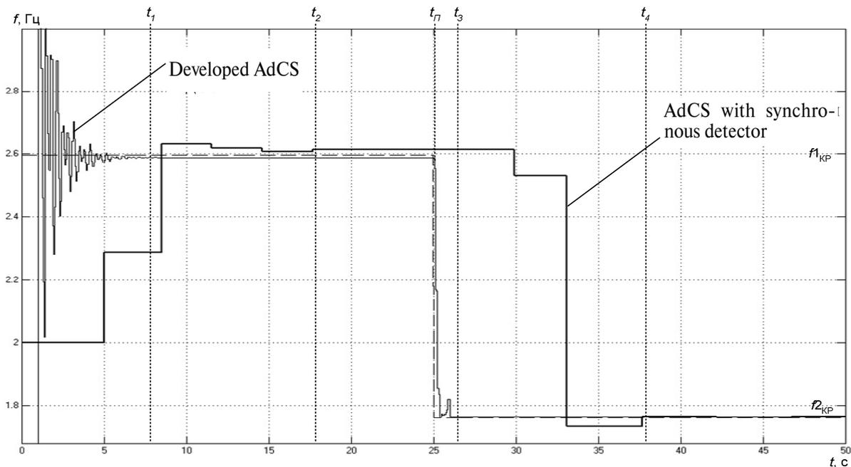
Fig. 4. The procedure of identification of an object by frequency technique
