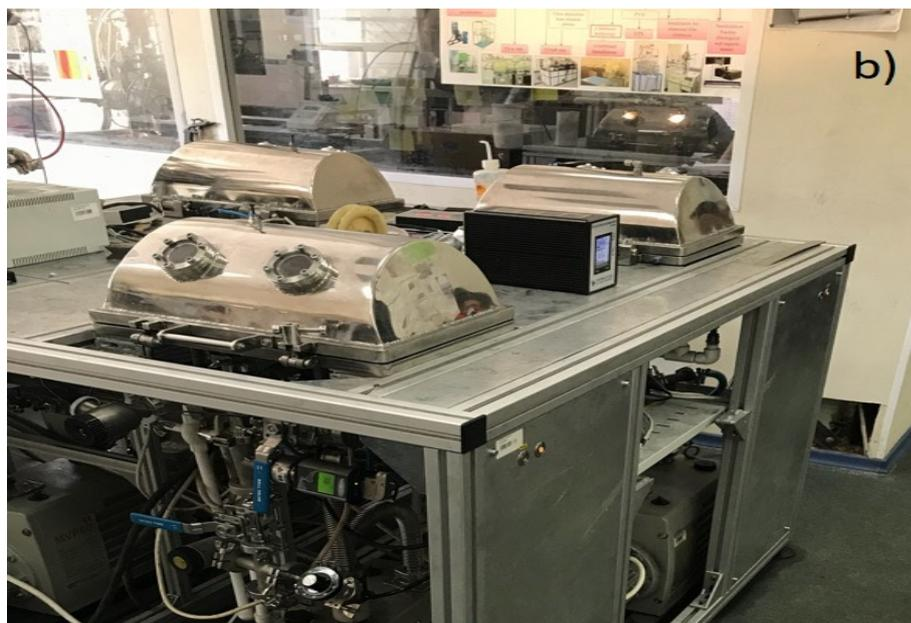
Figure – 2.5 Scheme of reactor (a) and general view of the HFCVD reactor (b): 1- gas supply; 2- gas distribution system; 3- tungsten filament; 4,5- fixation and tension system; 6- substrate; 7- pumping out
