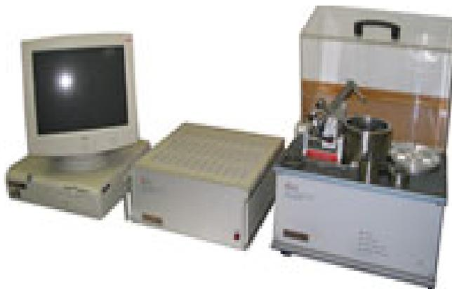
Figure 2.8 - High Temperature Tribometer (PC-Operated High Temperature Tribometer THT-S-AX0000)
