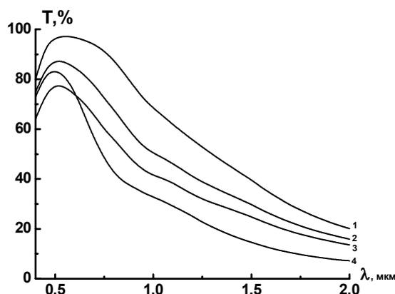
Fig. 4. Spectral transmittance index  $\text{TiO}_2\text{-Ag-TiO}_2$  (1, 3) and  $\text{SnO}_2\text{-Ag-SnO}_2$  (2, 4) with one (1, 2) and two (3, 4)  $\text{Ni}_{85}\text{Cr}_{15}$  protective layers
