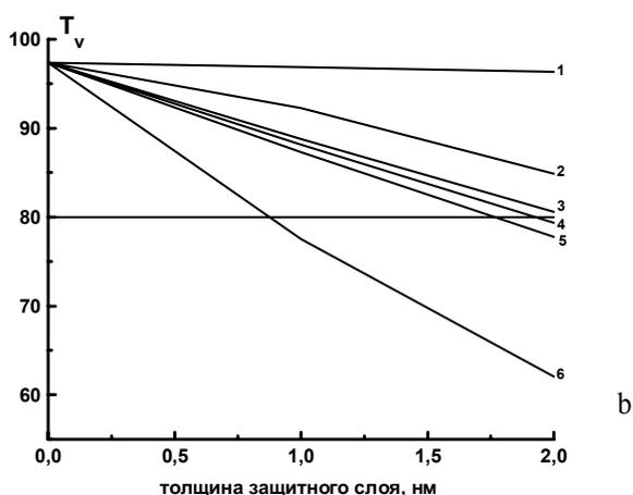
Fig. 3. Influence of protective layer thickness on visual transmittance index  $\text{TiO}_2\text{-Ag-TiO}_2$  (a) and  $\text{SnO}_2\text{-Ag-SnO}_2$  (b). For different materials: 1) Si, 2) Al, 3) Ti, 4)  $\text{Ni}_{85}\text{Cr}_{15}$ , 5) Ni, 6) Cr
