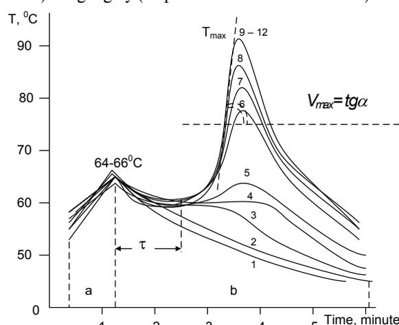
**Fig. 1.** Temperature change in time at aluminium nanopowder and water interaction: a) simultaneous heating and stirring of suspension; b) only stirring of suspension;  $\tau$  – breakdown time, min;  $V_{\max}$  – maximal rate of temperature rising, °C/s;  $T_{\max}$  – maximal value of suspension (water) temperature; 1,2,...,12 – suspensions numbers with various aluminium content (table)
