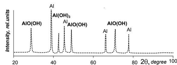
**Fig. 3.** X-ray of aluminium nanopowder and water interaction product in suspension of sample № 12 (table)
