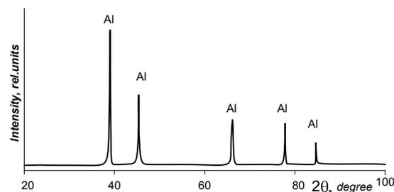
**Fig. 2.** X-ray of electroexplosive aluminium nanopowder
