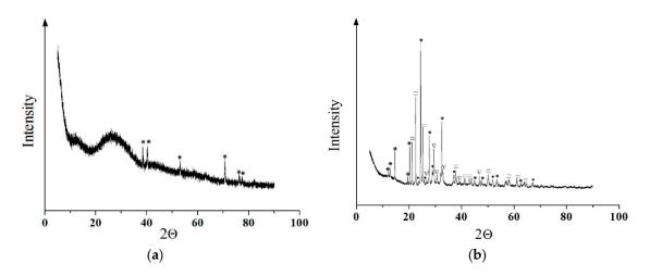
**Figure 3.** Diffractograms of the CP coating on a titanium surface obtained using the microarc oxidation (MAO) method. (a) The amorphous halo from the CP coating and the peaks from the titanium substrate; (b) the calcium phosphate coating after annealing at 1073 K. Peaks correspond to the phases:  $*-\text{CaTi}_4(\text{PO}_4)_6$ ,  $\Box-\text{TiP}_2\text{O}_7$ ,  $\bigtriangledown-\beta-\text{Ca}_2\text{P}_2\text{O}_7$ , and  $\bullet-\text{TiO}_2$  (anatase).
