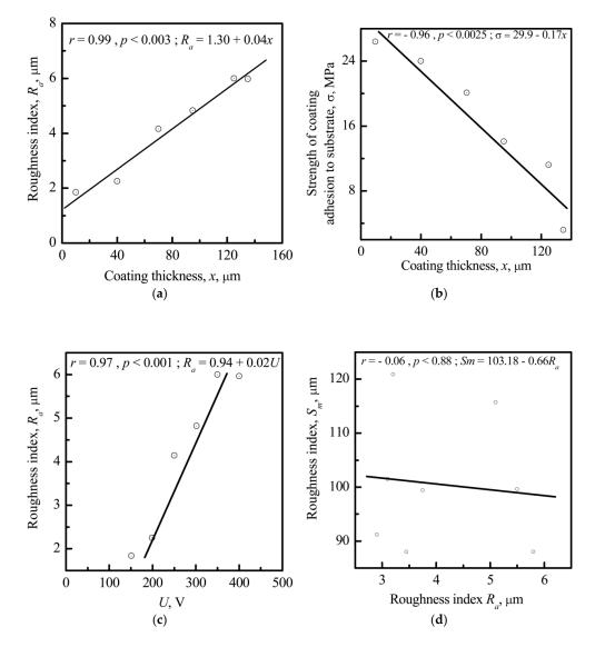
**Figure 8.** Correlations between (**a**) the CP coating thickness (x) and the roughness index  $R_a$ ; (**b**) the CP coating thickness (x) and the adhesion strength of the CP coating to the metal substrate; (**c**) the amplitude of the electrode voltage (U) of the microarc device and the roughness index  $R_a$ ; and (**d**) the CP roughness indices  $R_a$  and  $S_m$ .
