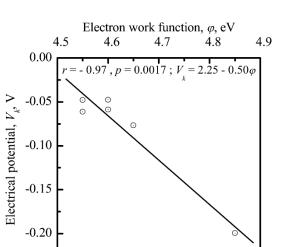
**Figure 14.** Relationship between the EP ( $V_k$ ) and the electron work function ( $\varphi$ ) of the CP surface at the nanoscale level.
