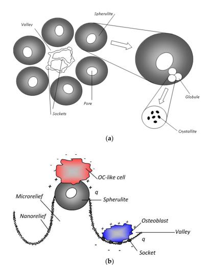
**Figure 17.** Schematic image of structural elements of the MAO CP coating (**a**) and nonuniform differentiation of cells in HLPSC culture (**b**). OC, osteoclast.
