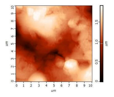
Figure 6. AFM image of the CP surface.
