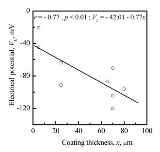
Figure 7. Correlation between the electrical potential (EP), V<sub>L</sub>, and the CP coating thickness, x.
