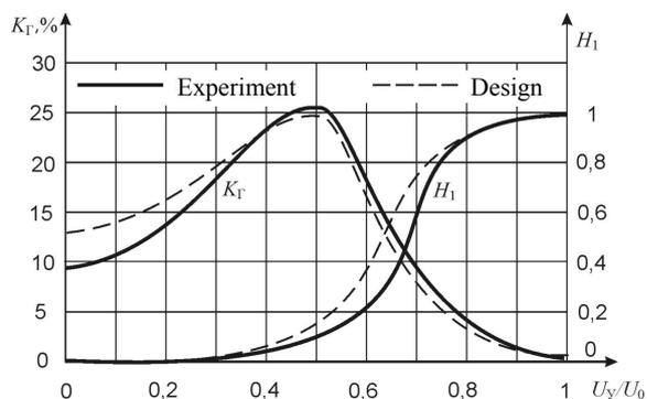
**Fig. 5.** Regulation curves and harmonic factor of attenuator with parallel MOSFET connection KP305 type in the conditions of constant output voltage  $u_{out}=100$  mV at frequency 1000 Hz
