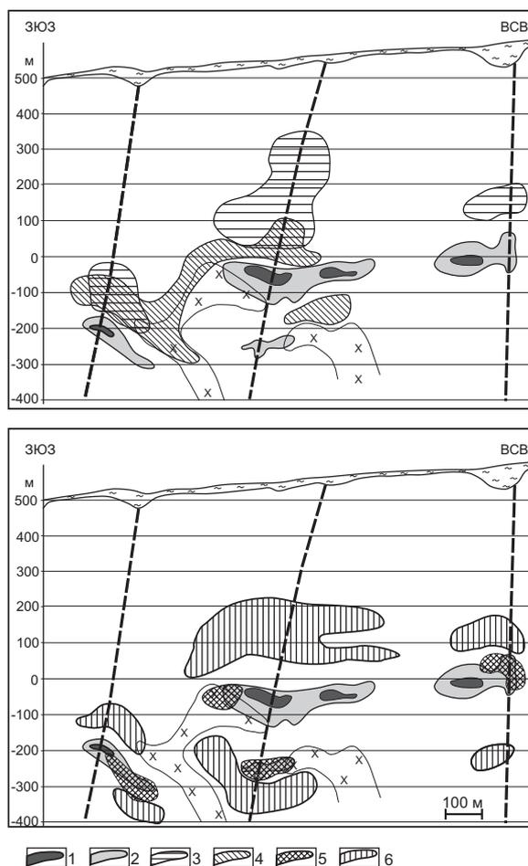
**Fig. 2.** Distribution of geochemical parameters anomalies in a cut through Southern Zone deposit of the Kazskiy ore field: 1)  $F1=0,36Ag+0,35Pb+0,28Cu+0,25Zn+0,23Au+0,19As$  ( $>4,8$ ); 2)  $F2=0,48Ni+0,46Cr+0,20Co$  ( $>3,0$ ); 3)  $F3=0,47Ba+0,42Mn$  ( $>2,4$ ); 4) Ti (more than 0,55 %); 5) OK Co:Ni (more than 12,0); 6) OK Pb:Zn (more than 50,0)
