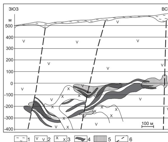
**Fig. 1.** Longitudinal geological section through Southern Zone of the Kazskiy ore field deposit (based on materials of «Tetis-T»): 1) Friable deposits; 2) the Sucharinskiy complex: andebasalts, calcitic and dolomitic marble; 3) diorites of the Telbesskiy complex; 4) skarn-magnetite ore deposits; 5) quartz-sulphidic mineralization zones; 6) explosive infringements
