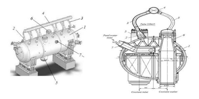
Figure 2.6- Exterior (a) and Cross section (b) of a horizontal steam generator: 1 - vessel; 2 - steam outlet nozzles; 3 - steam pipes; 4 - steam collector; 5 - input collector of the coolant; 6 - output collector of the coolant; 7 - pipe feed water
