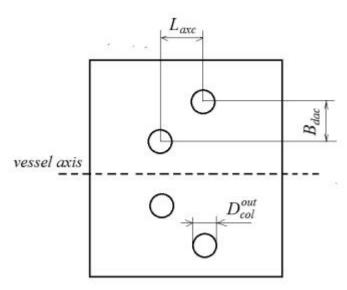
Fig. 2.8- To the calculation of the strength coefficient
