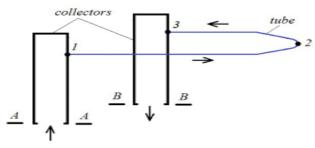
Figure 2.9- Flow diagram of the coolant circulation in a horizontal steam generator
