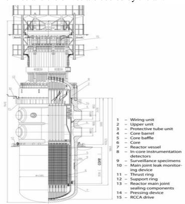
Figure 1.1- Reactor Design
