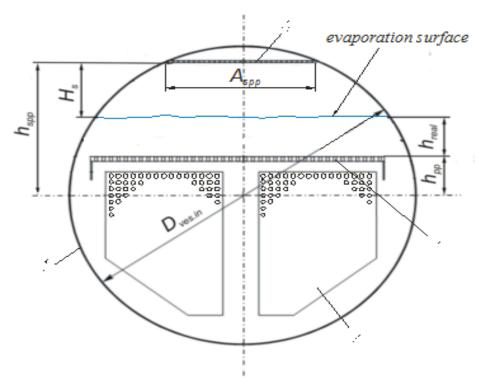
Figure 2.10- To the calculation of separation
