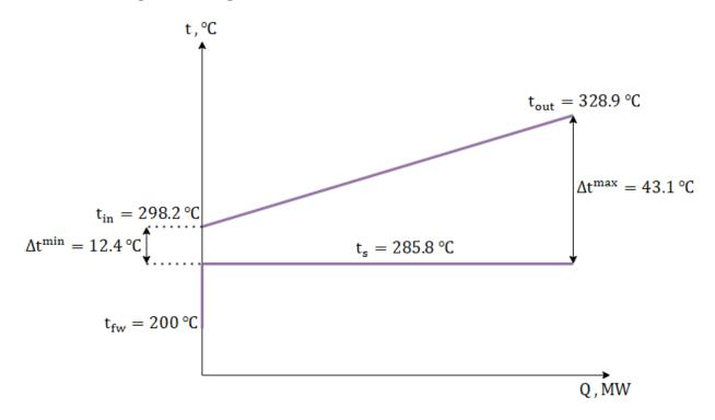
Figure 2.2- tQ-Diagrams of the Steam Generator
