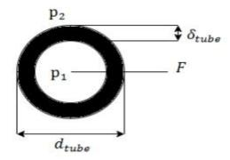
Figure 2.3- Cross Section of Heating Surface
