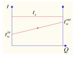
Figure 3.4- To the calculation of the logarithmic temperature difference  $\bar{\Delta t}$  is logarithmic temperature difference, °C
