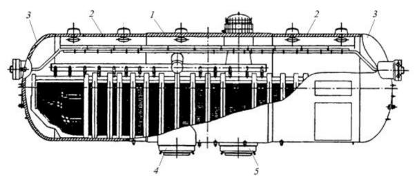
Figure 2.7- Longitudinal section of a horizontal steam generator:
