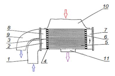
Figure 4.1- To the hydraulic calculation of the condenser
