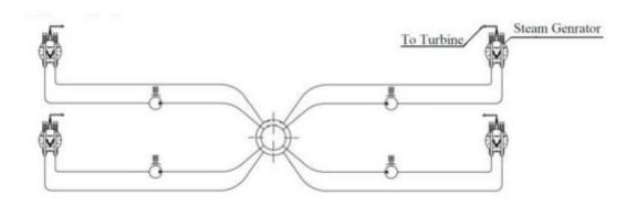
Figure 1.3- Primary Circuit Components of VVER-1200 (for 4 Loops)
