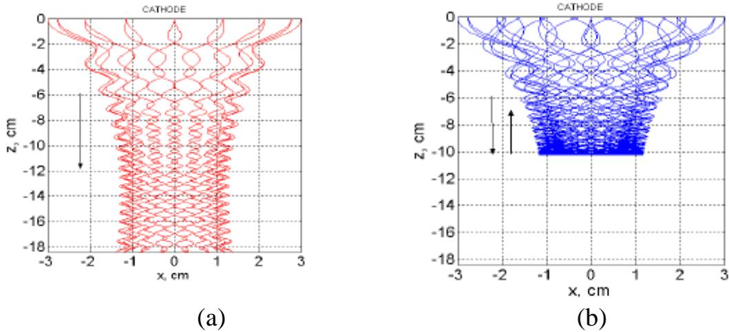
Figure 2.2. (a) Electron beam compression; (b) Pinch effect
