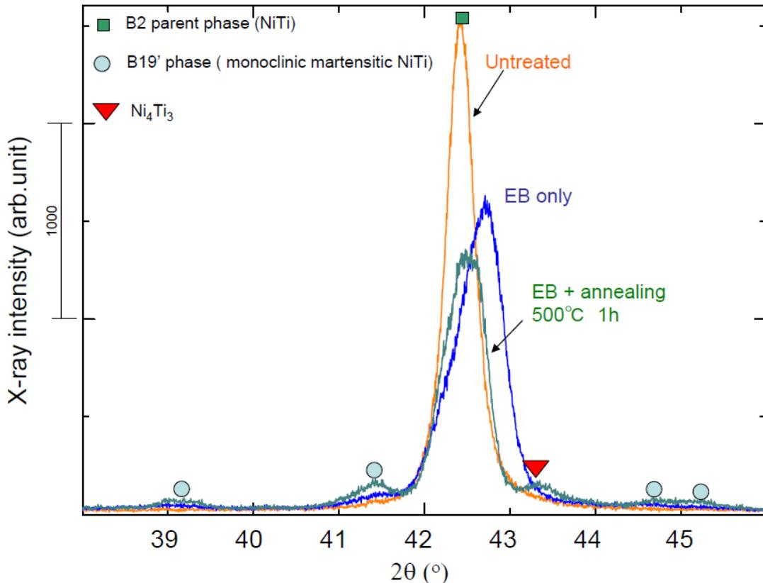
Figure 3.3. Intensity of  $Ni_4Ti_3$  in NiTi samples after treatment by the electron beam and annealing
