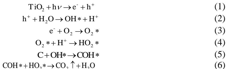
Titanium dioxide in combination with nitrogen when adding pure titanium dioxide ( $\text{TiO}_2/\text{TiO}_{2-x}\text{N}_y$ ) has a higher photo-catalytic activity than anatase (see Fig. 3.7).
