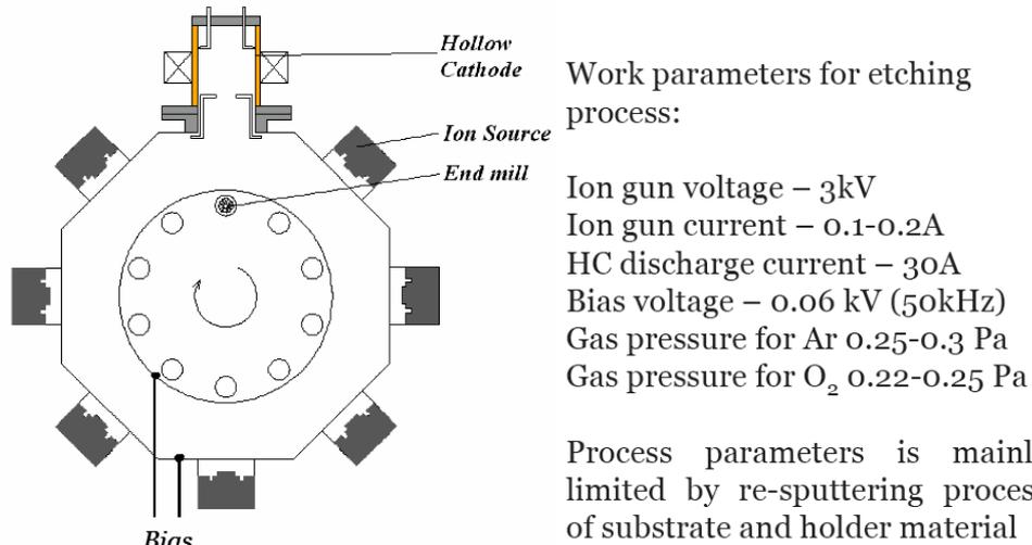
Figure 2.7. Combined system of Ion Guns and Hollow Cathode. The main parameters are shown in right sides
