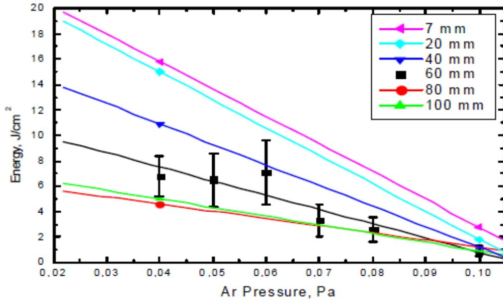
Figure 2.3. Dependence of energy of the electron beam on argon (the distance from electron gun to the calorimeter is given in Figure)
