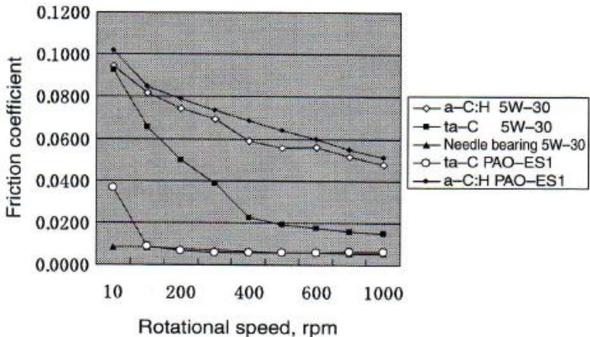
Figure 1.2. The dependence of the friction coefficient on rotational speed
