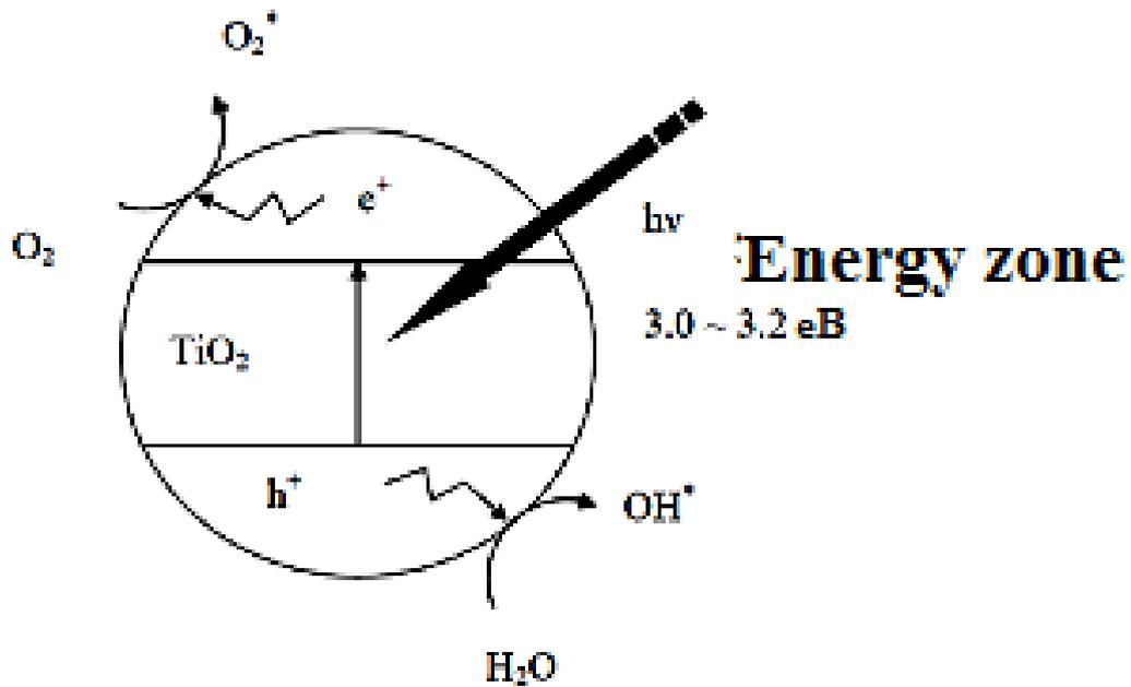
Figure 3.6. The reaction mechanism of photo-catalysis using  $\text{TiO}_2$
