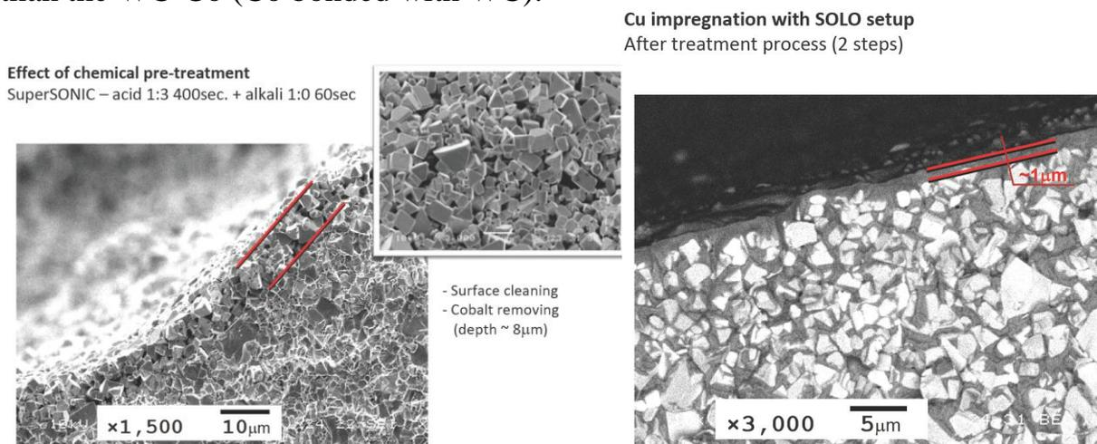
Figure 3.1. The microstructure of the die filter after the deposition of copper
