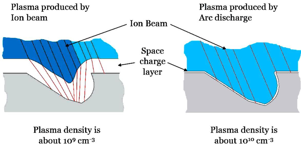
Figure 2.6. Space charge layer dimension is inversely proportional to the plasma density especially in case of complex shape
