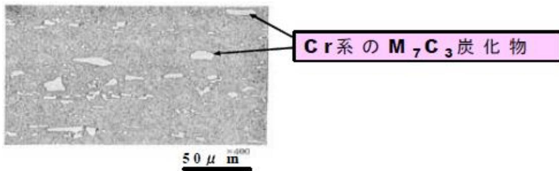
Figure 3.2. The microphotograph of the SKD11 steel. The arrows indicate the inclusion of metal carbide with chromium
