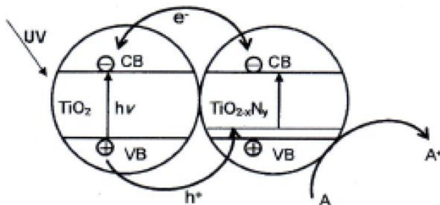
Figure 3.7. The scheme of the photon induced charge separation on the compound of  $\text{TiO}_2/\text{TiO}_{2-x}\text{N}_y$
