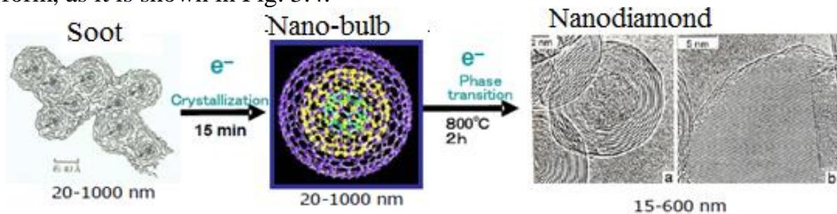
Figure 3.4. The scheme of formation of the nano-diamonds from nano-carbon bulbs
