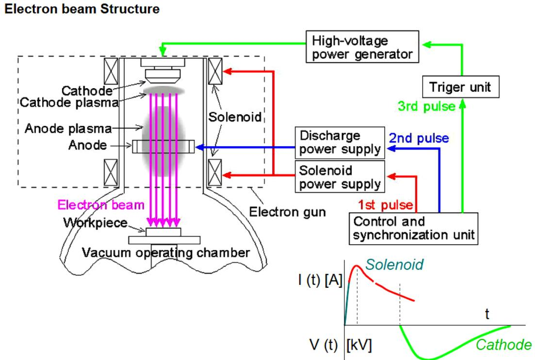
Figure 2.1. The scheme of the setup intended for generation of the electron beam [1]
