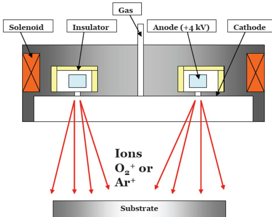
Figure 2.5. Scheme of Ion Gun
