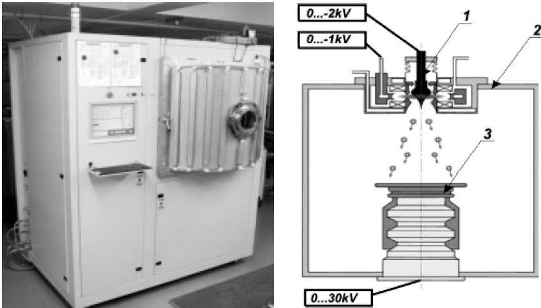
Figure 2.8. The picture of the setup for the ion implantation and the scheme the setup. 1 - Ion gun on the base on target sputtering by Penning discharge plasma, 2 – vacuum chamber, 3 - samples holder on thebase insulator
