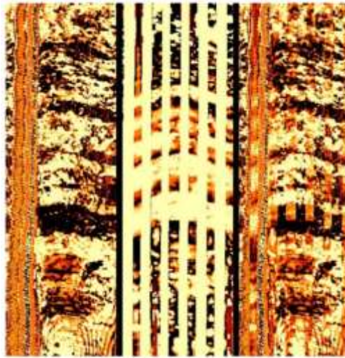
Figure 2.2 – Images show CBIL (left), Earth Imager (middle), and merged (right) for a same 10-ft interval [48]
