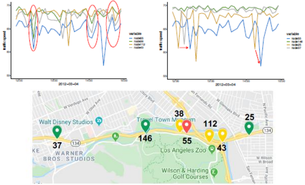
Figure 7: Case study (a — Time series of node 55 and its top-3 neighbors given by the pre-defined A, b — Time series of node 55 and its top-3 neighbors given by the learned A, c — Node locations of node 55 and its neighbors marked on Google Maps. Yellow nodes represent node 55’s top-3 neighbors given by the pre-defined A. Green nodes represent node 55’s top-3 neighbors given by the learned A.)
