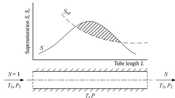
Fig. 1. Change of vapor flow supersaturation degree when moving along the tube
