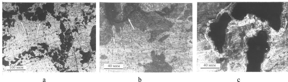
Fig. 2. Microstructure of steel St52,3N of waste blank: a) general view of microstructure, pores are indicated with arrows; b) fine structure of pearlite colony, chain of pores is indicated with arrows; c) pores in pearlite colony
