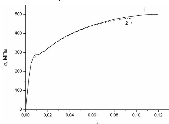
Fig. 1. The diagram of steel St52,3N samples loading
