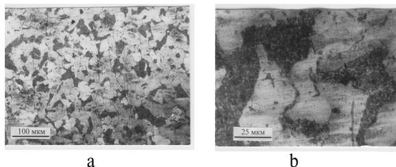
**Fig. 3.** Microstructure of steel St52,3N of conditional product: a) general view of microstructure; b) fine structure of pearlitic colony
