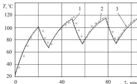
**Figure.** The time change of betatron winding peak temperature in the point  $X=0,5$ : 1) exact analytical solution; 2) approximate calculation; 3) experimental data [3]
