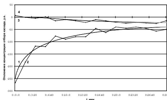
**Fig. 3.** Time dependence of concentration deflection of selection cascade with respect to reference quantity in standard units (1 s.u.=0,001 %). Closing steps: 1) calculation; 2) real – selective and 3) calculation; 4) real – predump
