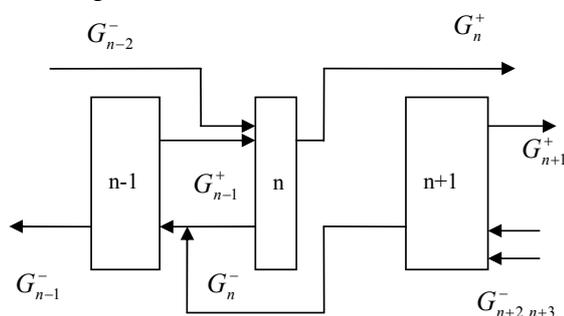
Fig. 2. Parallel-series circuit of step connection in cascade
