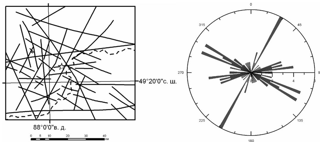
**Fig. 4.** The scheme of lineaments of the Kalgutinskiy deposit area and their rose-diagram. The frontier is hereinafter shown by a dashed line
