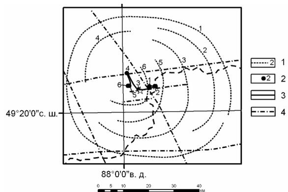
Fig. 6. Cosmostructural model of the Kalgutinskiy deposit area: 1) basic ring structures and their numbers, 2) centroids of ring structures and their number, 3) projection onto the day time surface of the trajectory of change of focus position of the Kalgutinskiy ore-magmatic system, 4) basic lineaments of the area
