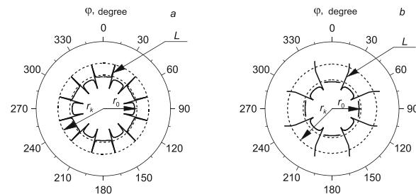
**Fig. 2.** Release boundary for betatron of type: a) MIB-6; b) MIB-1
