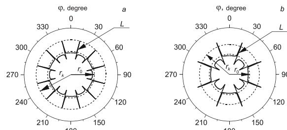
**Fig. 1.** Boundary of release for betatrons of the type: a) MIB-6; b) MIB-1; L is the boundary of release
