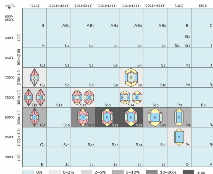
Figure 15. Quantitative distribution of zircon grain morphotypes from tonstein I-12 according to the diagram of Pupin [70]; morphotypes S18 and S19 with developed prismatic facets {100} predominate.
