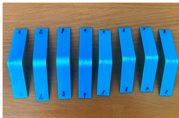
Figure 9. Photos of the specimen bending after mechanical testing.
