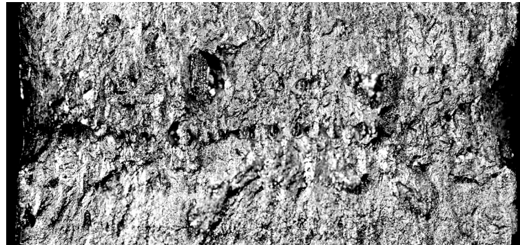
Figure 4. Fractogram of the fracture site in the zone of destruction retardation under cyclic loading (tightening of the cross-section of a compact sample); \times 4 .
