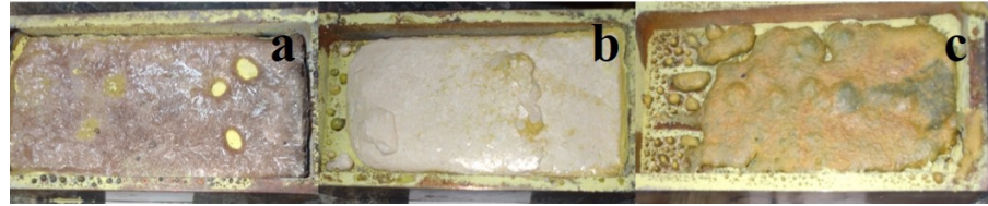
Figure 10. Photographs of ceramic samples (a) ZnWO 4 , (b) MgWO 4 , (c) CaWO 4 , synthesized under the influence of an electron beam with E = 1.4 MeV, P = 18 kW/cm 2 , R1.
