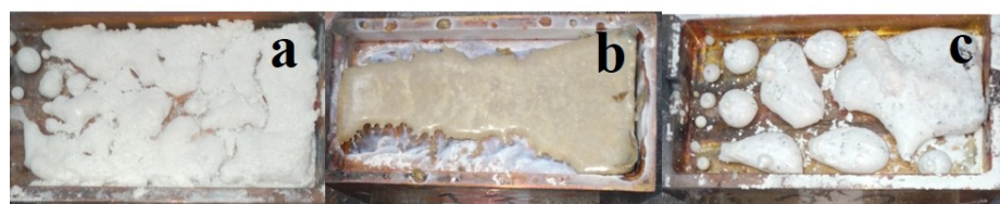
Figure 7. Photographs of activated W samples of BaF 2 (a), MgF 2 (b), and BaMgF 4 (c) ceramics synthesized under the influence of an electron beam with E = 1.4 MeV, P = 15 kW/cm 2 , R1.
