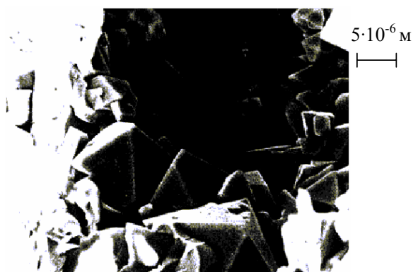
Fig. 5. Particles of aluminum and iron oxide in reaction product structure in the system of alloyed steel scale – aluminum
