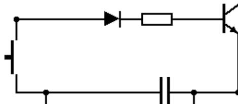
2) Base open. Juice flows through the condenser and resistor, It is charged.
