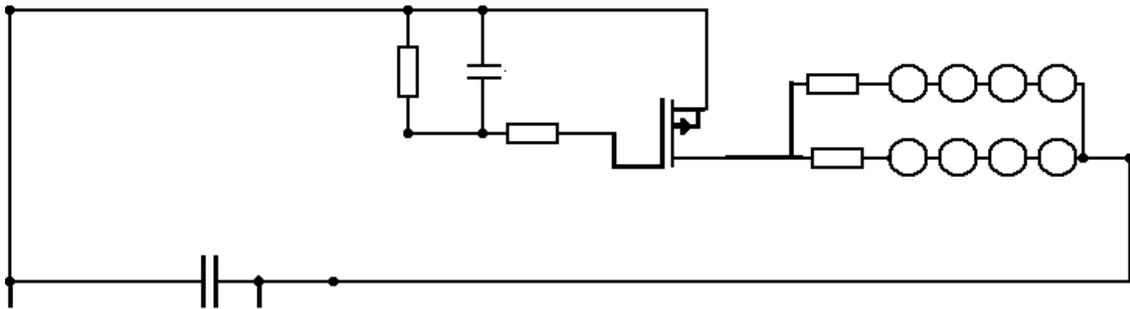
Group of LEDs vary in capacitance of the capacitor and the resistance of the resistor. it regulates time of the work of LEDs
