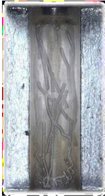
Figure 2. Stroboscopic image of pellet movement in annulus space.
