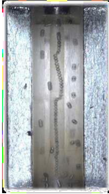
Figure 3. Stroboscopic image of pellet movement in the drill bit.
