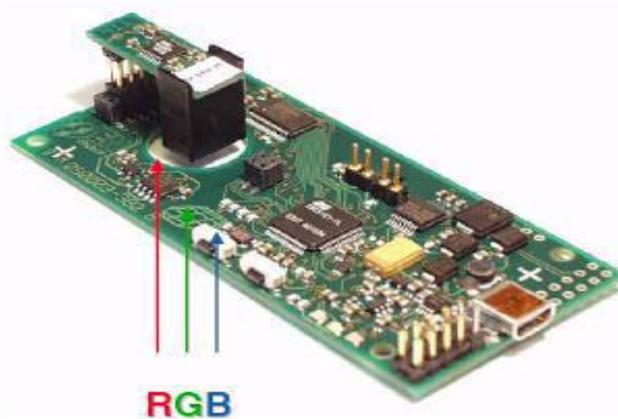
Figure 4. Evaluation Board for determining the color coordinates
