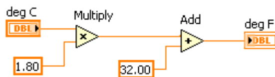
Figure 2.6 – An example program on LabVIEW. Celsius to Fahrenheit conversion.
