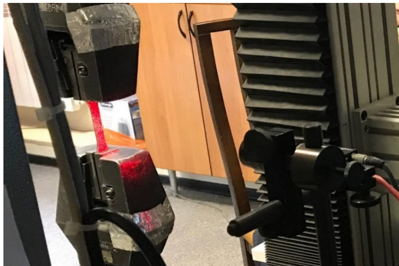
Figure 8. Survey of spectrographs using the DIC method
