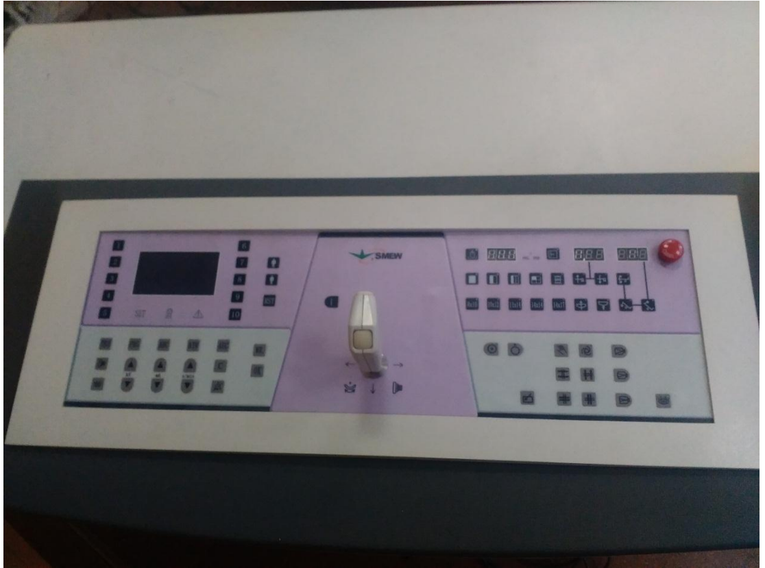
Fig3.3. Long distance control panel.
