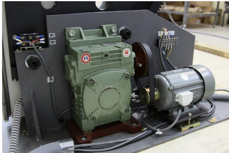
Fig.2.7. AC motor and Mechanical systems for Bed rotation
