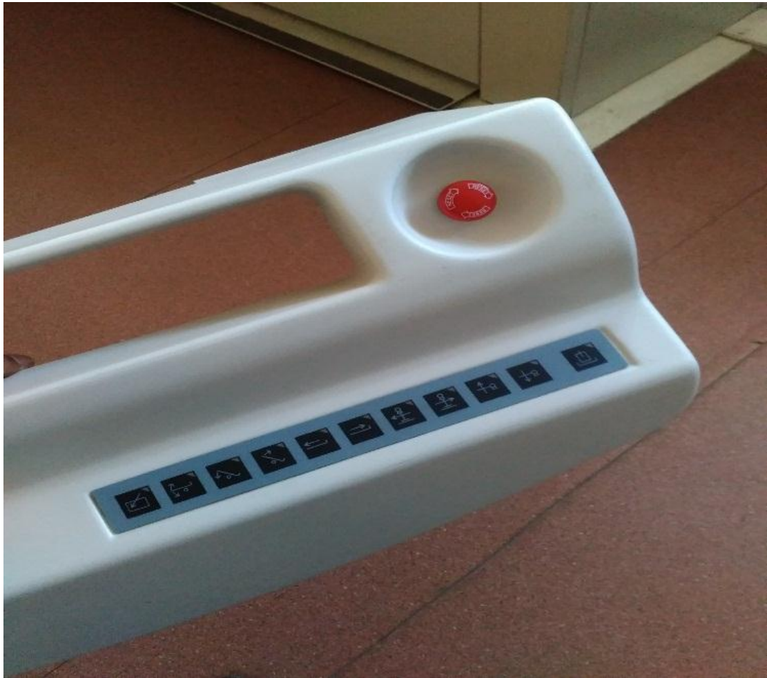
Fig.3.3. Short distance control panel.
