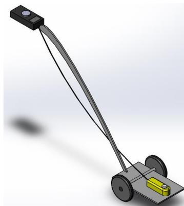
Picture 1.2. "Cart transportation" for illumination measurement
