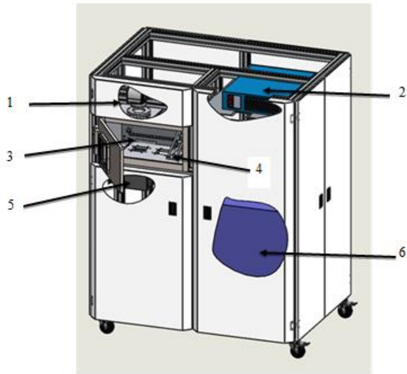
Figure 11. Project of the developed setup for SLS printing
