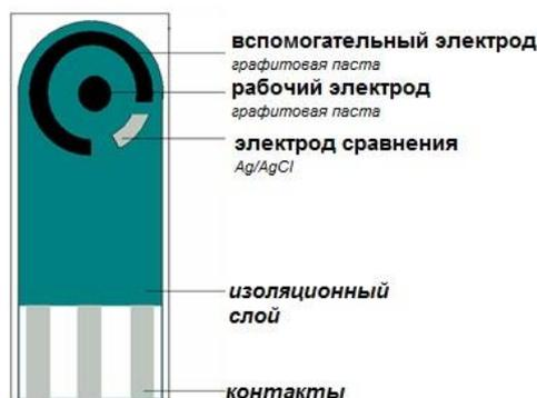
Figure 5. Physical configuration of the electrode produced by screen printing method
