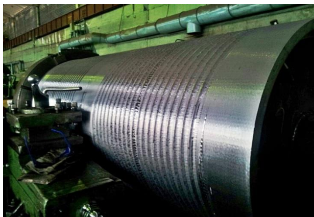
Figure 1.3-cutting grooves on the drum in the workshop of the PMZ
