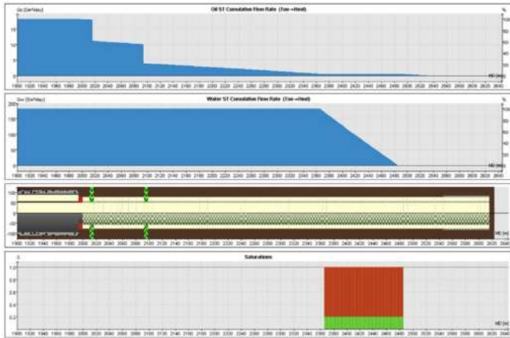
Figure 1.3 - Simulation of a water cone breakthrough with a well equipped with a screen (Sleptsov, 2019)
