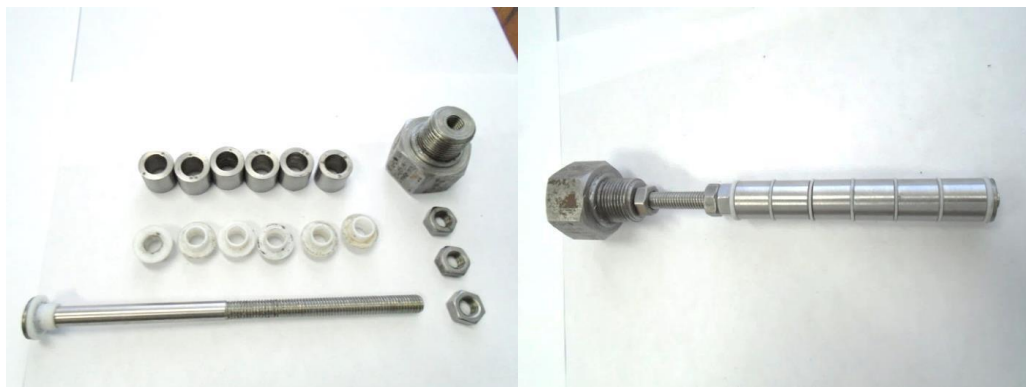
Figure 4 - Typical gravimetric cassette with 6 samples
