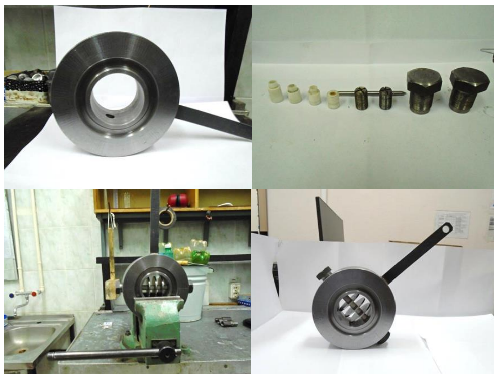
Figure 5 - Corrosion rate control assembly
