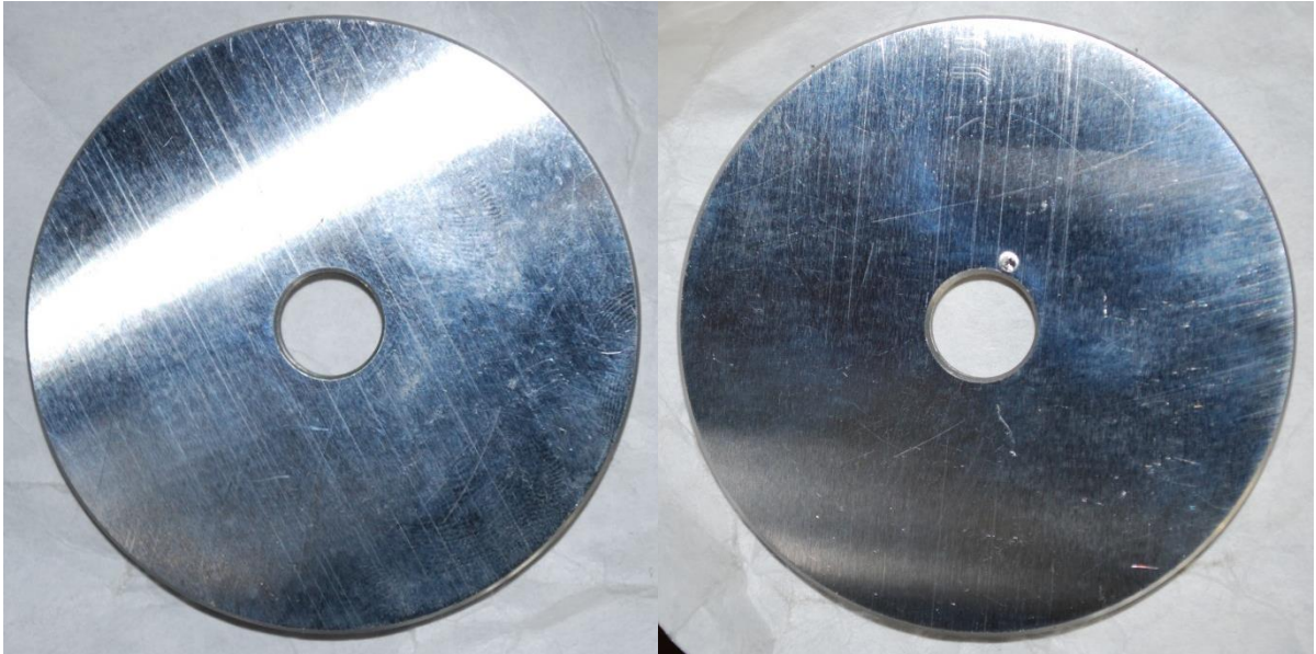
Figure 7 - Prepared corrosion witness samples
