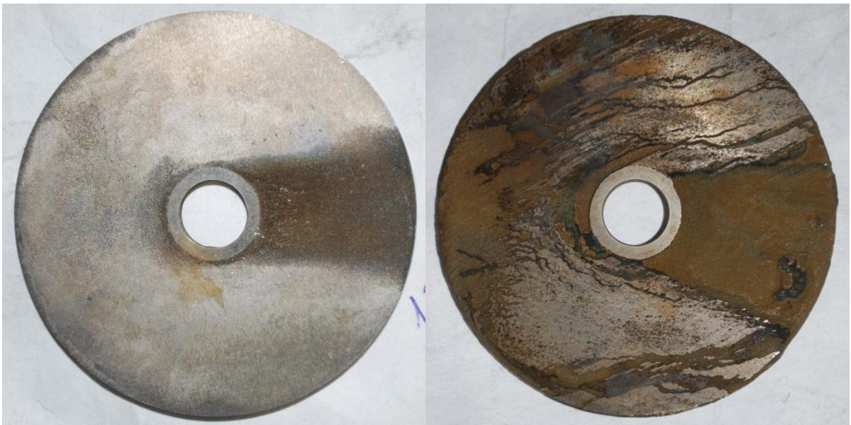
Figure 8 - Corrosion witness samples after exposure to the medium
