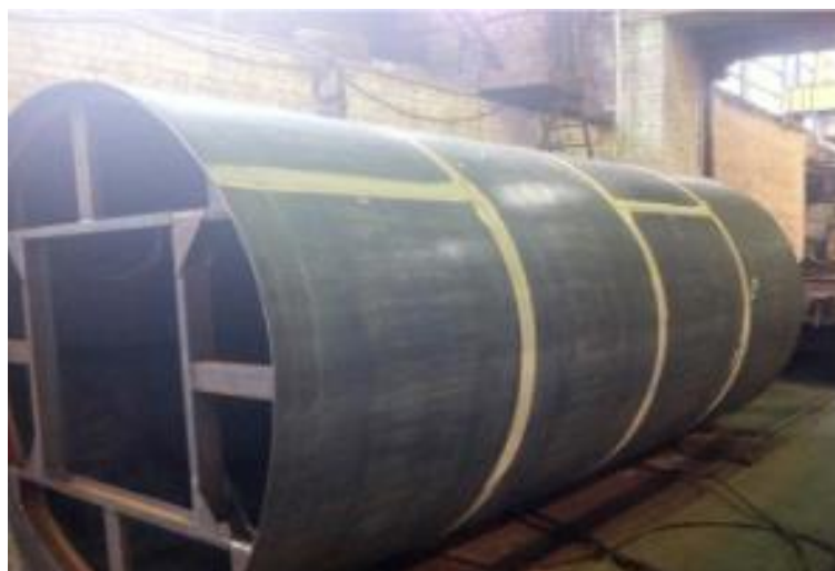
Figure 2 – Prepared roll for the tank wall
