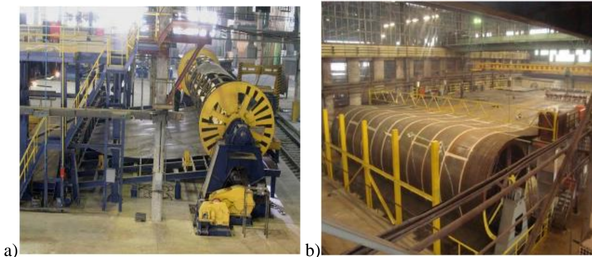
Figure 4 – Rolling stands: a) one-tier stand, b) two-tier stand
