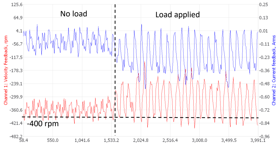
Figure 4.7 - Reading of the stator current's q -component (blue) and the rotation speed (red) of the PMSM at -400 rpm (attaching load)
