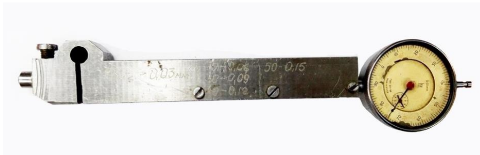
Fig. 6. Mandrel with flat spring hinge type.
