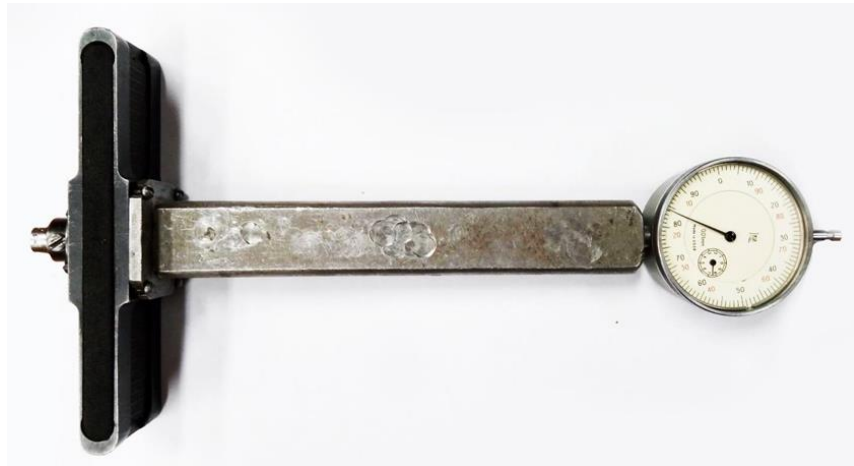
Fig. 7. Diamond blade with flat symmetrical spring
